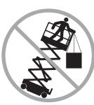
Do not place or attach fixed or overhanging loads to any part of this machine.
