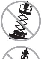
Do not raise the platform unless the machine is on a firm, level surface.
